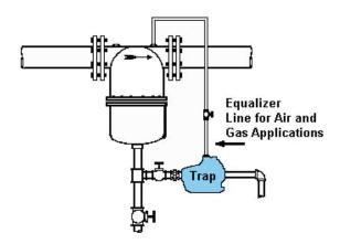
Just as steam separators and steam traps work together to optimize a steam system, we work with YOU to properly size separators and traps for your specific application. Call us at 908.362.9981 or use our inquiry form for immediate assistance with your application!
