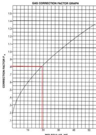
Let's walk through an example for natural gas of consisting 75% Methane (CH<sub>4</sub>: 16 MW) and 25% Nitrogen (N2: 28 MW). The design (maximum) pressure is 120 PSIa and the temperature is 90°F. Our design (maximum) flow rate is 1,000 lbs/hr.
