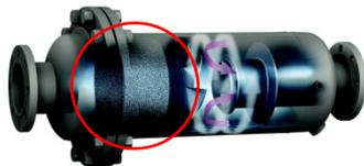
It is possible to remove droplets smaller than 1 micron with the addition of a filter element stage after the separation stage. These specially designed borosilicate microglass filter elements have a glass matrix drainage layer in support of retentions as fine as 0.30 microns.
