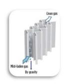
vane includes pathways to isolate the separated liquid from reentrainment into the process gas.
