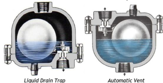
In conclusion, while float drain traps offer simplicity and reliability, inverted bucket traps excel in managing oil contamination and recovering steam. The choice between the two depends on the specific requirements of the application. Whether it's steam or compressed air systems, selecting the right drain trap is essential for efficient condensate removal and system performance.
