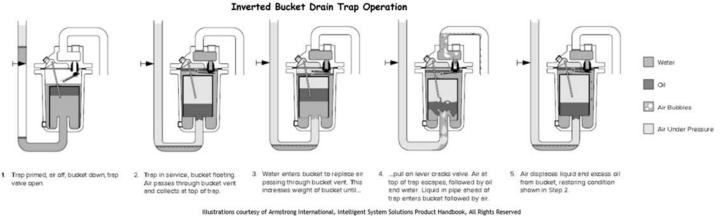
**Inverted Bucket Traps** also operate on the principle of buoyancy although their mechanical design is more complex than a float drain trap. Inverted bucket drain traps are mostly used in steam systems although they can be used in compressed air and industrial gas systems
