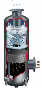
vessel itself has to be designed to provide access to the media for replacement.
