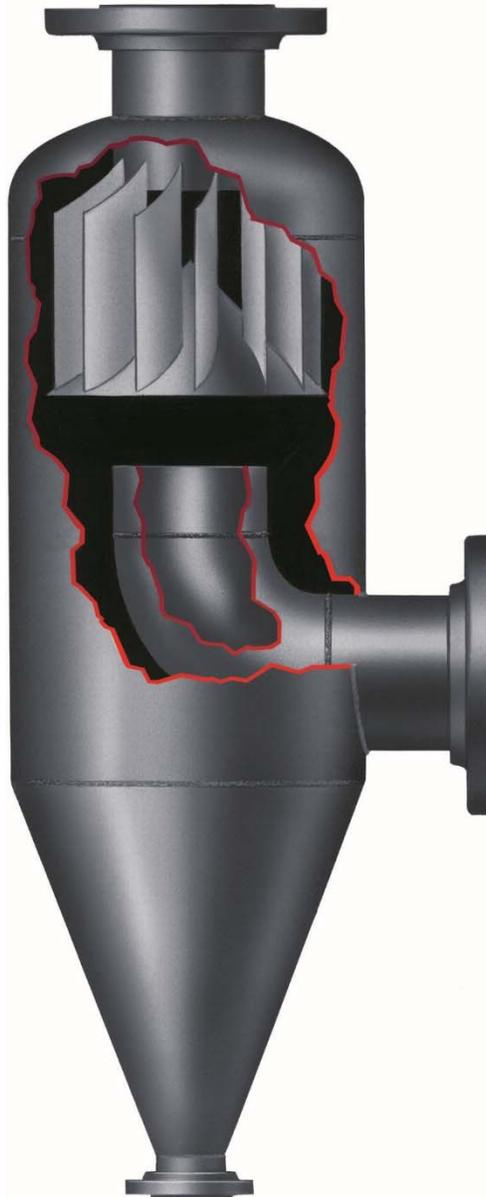
The centrifugal rotary motion causes the entrained droplets and particles to rotate away from the center of rotation, thus to the outer walls of the vessel. The larger size droplets with a heavier mass are forced to the outer wall first and the finer (lower mass) droplets take longer to impinge onto that surface. A degree of angular momentum assists with separation although it is not the primary separation mechanism.
